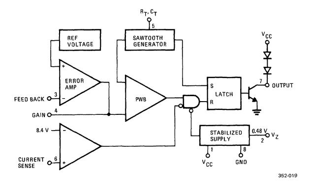
Figure 5-4. Simplified Series-Pass Pulse Width Modulating Regulator
